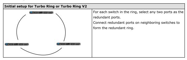
The user does not need to manually assign the master with Turbo Ring or Turbo Ring V2. If no switch is assigned as the master, the protocol automatically selects one of the switches to be the master. The master is only used to identify which segment in the redundant ring acts as the backup path. In the following subsections, we explain how the redundant path is selected for rings configured for Turbo Ring and Turbo Ring V2.
