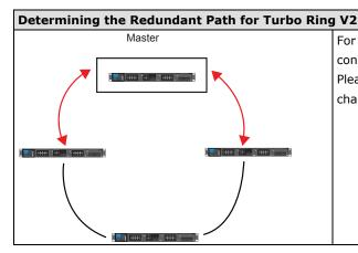
For Turbo Ring V2, the backup segment is the segment connected to the 2nd redundant port on the master. Please refer to Configuring Turbo Ring V2 later in this chapter.
