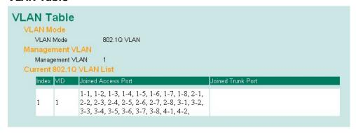
In 802.1Q VLAN table, you can review the VLAN groups that were created, Joined Access Ports, and Trunk Ports, and in Port-based VLAN table, you can review the VLAN group and Joined port.
