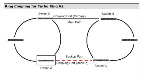
Note that the ring coupling settings for a **Turbo Ring V2** are different from a **Turbo Ring**. For Turbo Ring V2, ring coupling is enabled by configuring the **Coupling Port (Primary)** on Switch B and the **Coupling Port (Backup)** on Switch A only. You do not need to set up a coupling control port, so **Turbo Ring V2** does not require a coupling control line.
