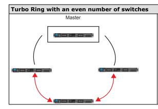
If the number of Ethernet switches in the Turbo Ring is 2N (an even number), the backup segment is one of the two segments connected to the (N+1) st switch (i.e., the unit directly opposite the master).
