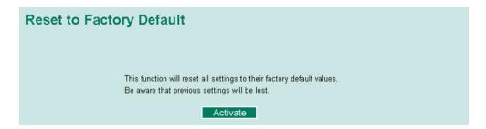
This function provides users with a quick way of restoring the IKS-6726-8PoE's configuration to factory defaults. This function is available in the serial, Telnet, and web consoles.
