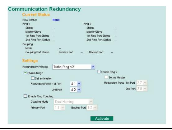
**NOTE** When using a dual-ring architecture, users must complete configuration for both Ring 1 and Ring 2. The status of both rings will appear under Current Status.
