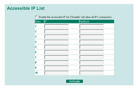
You may add or remove IP addresses to limit access to the IKS-6726-8PoE. When the accessible IP list is enabled, only addresses on the list will be allowed access to the IKS-6726-8PoE. Each IP address and netmask entry can be tailored for different situations:
