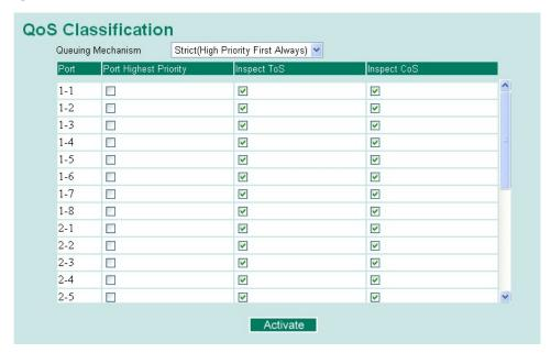
The IKS-6726-8PoE supports inspection of layer 3 TOS and/or layer 2 CoS tag information to determine how to classify traffic packets.
