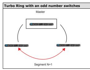
If the number of Ethernet switches in the Turbo Ring is 2N+1 (an odd number), the backup segment is the (N+1)st segment counting counterclockwise. For the example shown here, N=1, so that N+1=2.
