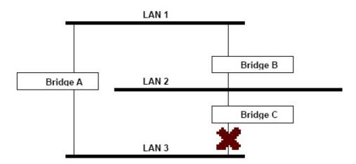
STP will determine which path between each bridged segment is most efficient, and then assign a specific reference point on the network. When the most efficient path has been identified, the other paths are blocked. In the above 3 figures, STP first determined that the path through Bridge C was the most efficient, and as a result, blocked the path through Bridge B. After the failure of Bridge C, STP re-evaluated the situation and opened the path through Bridge B.
