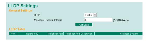
From the switch's web interface, users have the option of either enabling or disabling the LLDP, as well as setting the LLDP transmit interval (as shown in the figure below). In addition, users are able to view each switch's neighbor-list, which is reported by its network neighbors. Most importantly, enabling the LLDP function allows Moxa's MXview to automatically display the network's topology as well as system setup details such asVLAN, and Trunking for the entire network.
