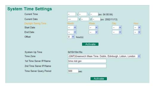
The IKS-6726-8PoE has a time calibration function based on information from an NTP server or user specified time and date. Functions such as automatic warning emails can therefore include time and date stamp.
